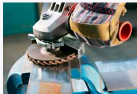
Quick, professional derusting and descaling
