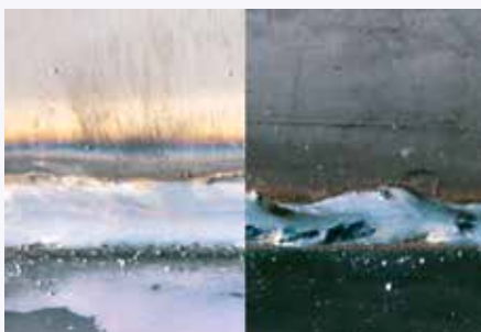
Surfaces descaled prior to welding result in clean welding seams (see image at left)
