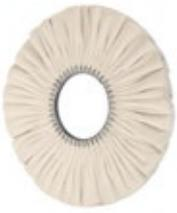
**Airflow Cloth Buff:** The standard ventilated buff, suitable for almost every step in the polishing process. Various qualities of grey cloth can be selected depending on the results required. The irregular folds fixed to a metal clinch ring, form a flexible and economical buff. Buffs can be used individually or mounted on a wide shaft, depending on the equipment available.
