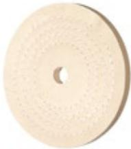
Discs of material are layered and stitched to a required width. Layers are arranged such that any fraying is minimal. By varying the grade of cloth and the stitching, different hardness's can be determined.
